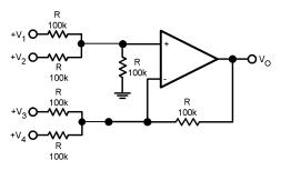
Where:  $V_0 = V_1 + V_2 - V_3 - V_4$ ,  $(V_1+V_2) \ge (V_3 + V_4)$  to keep  $V_0 > 0$   $V_{DC}$
