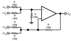
Where:  $V_0 = V_1 + V_2 - V_3 - V_4$ ,  $(V_1 + V_2) \ge (V_3 + V_4)$  to keep  $V_0 > 0$   $V_{DC}$
